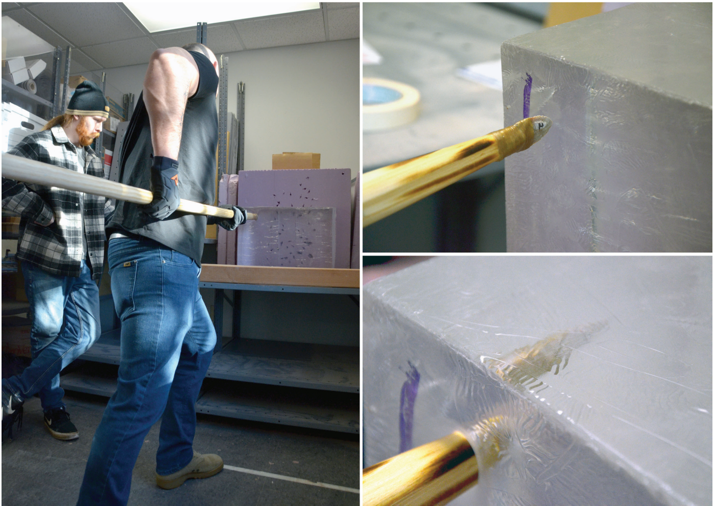
Figure 3. Left: Taylor thrusts a spear into ballistic gel while McKinny times how long the thrust should be sustained. Right: a spear before (above) and after (below) being thrust into the ballistics gel block.
