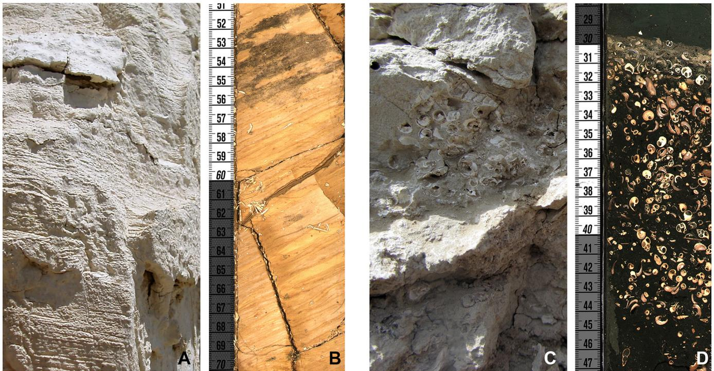
**Figure 10.** Comparison of outcrop versus drill core preservation. Close-up of diatomite outcrop adjacent to drilled Tugen Hills sequence (A) and laminated diatomite from BTB13-1A (B). Close-up of coquina adjacent to drilled West Turkana sequence (C) and coquina from WTK13-1A (D). Note that outcrop examples may not reflect exact correlates of drill core examples.
